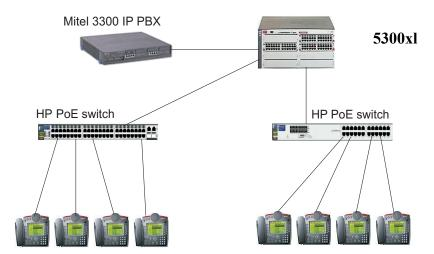
Figure 1-1. Example of a Typical Implementation
